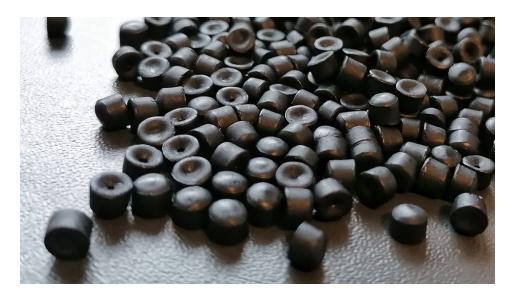
Granulated plastic made from net pens recycled in Norway. "Net pens have been recycled in Norway for decades, but this has primarily been synonymous with heat recycling in which the pens are granulated and the granulate burned in a special power plant," said Arnstein Hosaas, innovation director at AKVA group. Photo by Oceanize.
