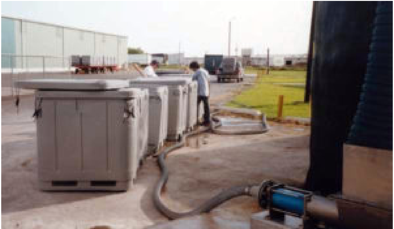
Prefilling totes with slurry ice can reduce harvest time. Photo courtesy of Sunwell Technologies Inc.
