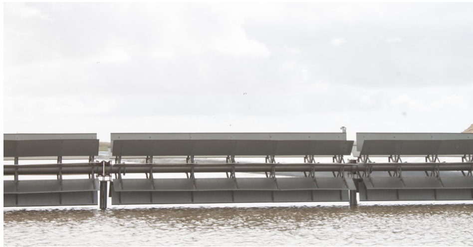
A view of the algae pond paddlewheels. Photo courtesy of Susewi.
