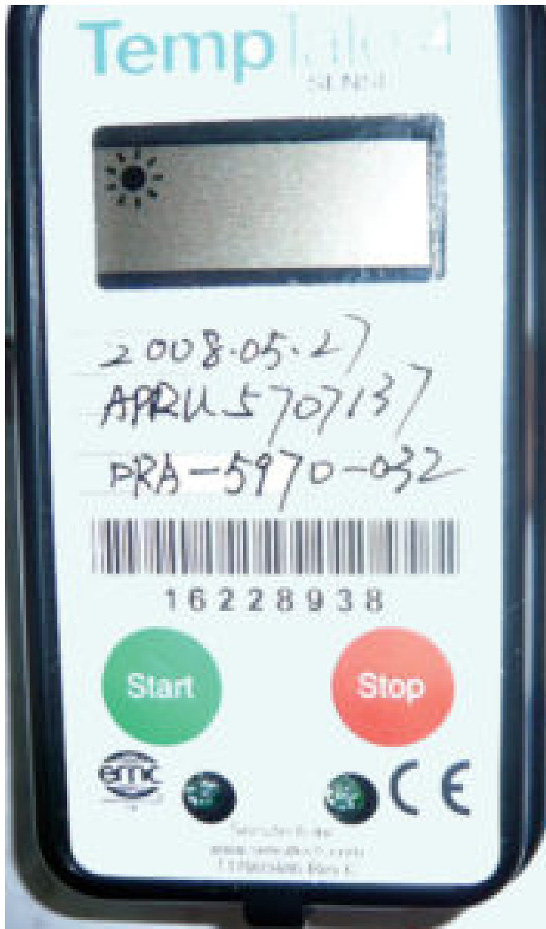
A typical temperature-recording device used in shipping containers. Photo courtesy of Sensitech Corp.
