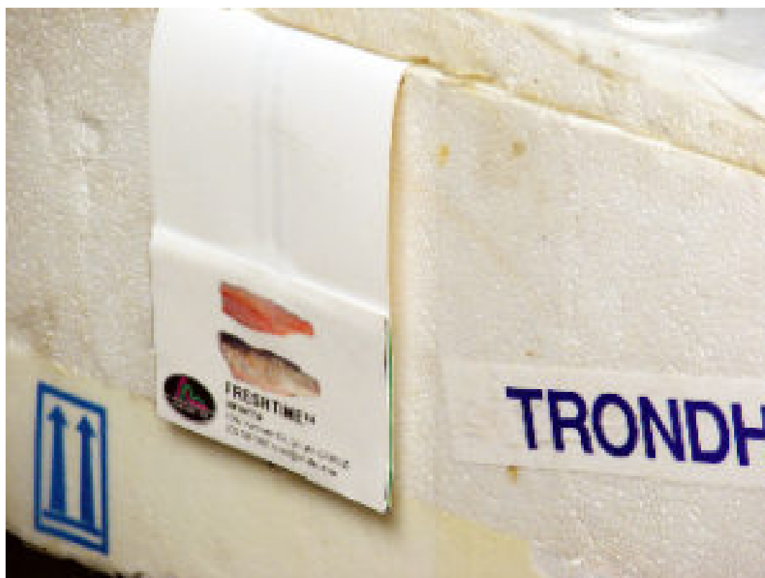
An RFID tag used to track products and temperatures in transit. Photo courtesy of Intrafab, Inc.
