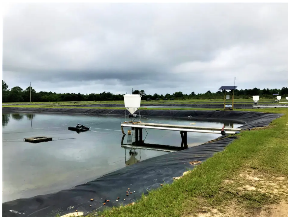
Fig. 1: Pond setup used in this experiment with solar powered AQ1 System between ponds. Each controller powered and managed two adjacent ponds.
