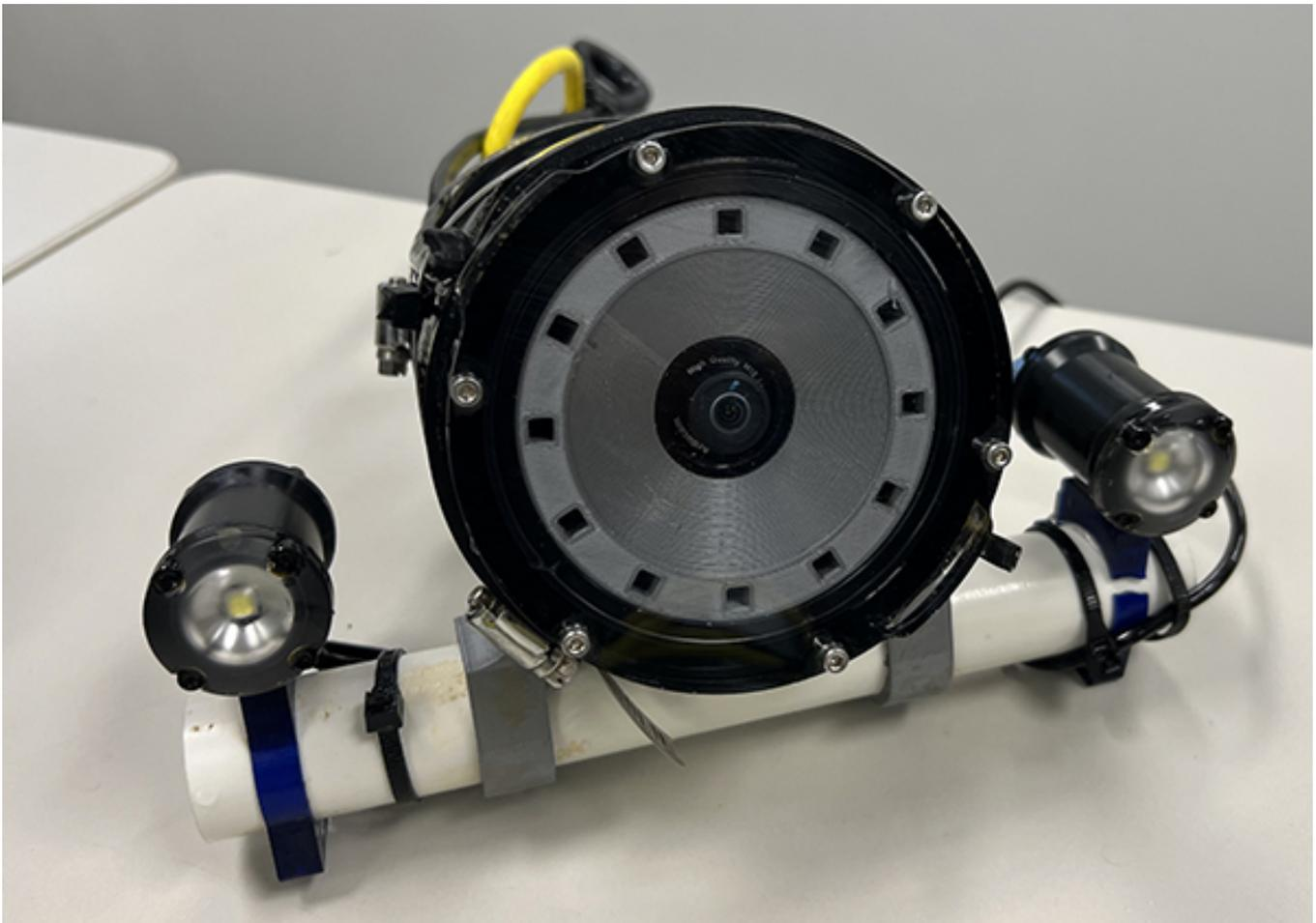
The MortCam (above) is a fish mortality monitoring and alert tool under development that can be deployed in recirculating aquaculture systems. Photo courtesy of the Conservation Fund.
