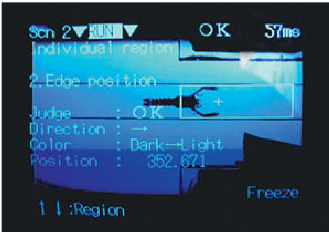
Image-processing software is used to identify molts, mortality, and harvest time.
