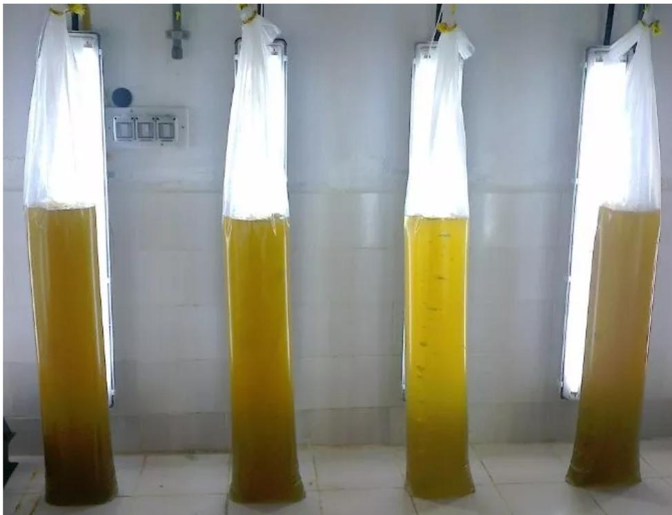
The best growing system for *T. weissflogii* is a cylindrical reactor with 110-m thick walls.
