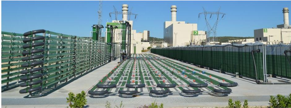
Photobiorreactors can be very efficient in removing nutrients and producing algal biomass. For example, 425 g N-  $\text{NH}_4^+$ /day and 125 g P- $\text{PO}_4^{3-}$ /day can be removed in large-scale wastewater remediation with photoautotrophic *Scenedesmus obliquus*. Wastewater phytoremediation with species such as *Chlorella* sp. can achieve 80 percent  $\text{NO}_3^-$  removal with a biomass yield of 160 mg/L/day. Photo of commercial facility in Spain by AlgaEnergy, via Wikimedia Commons.
