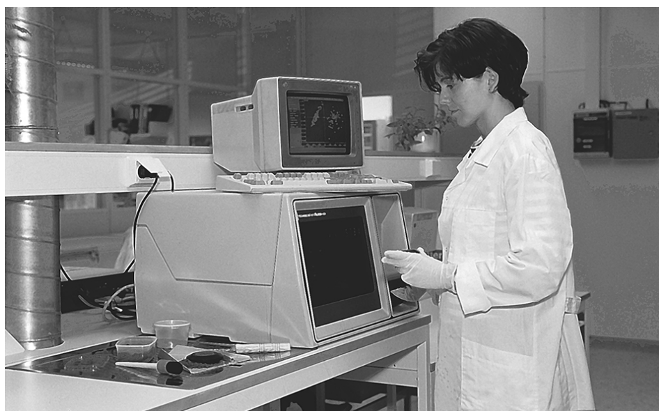
Analyzing feed composition using near-infrared reflectance.
