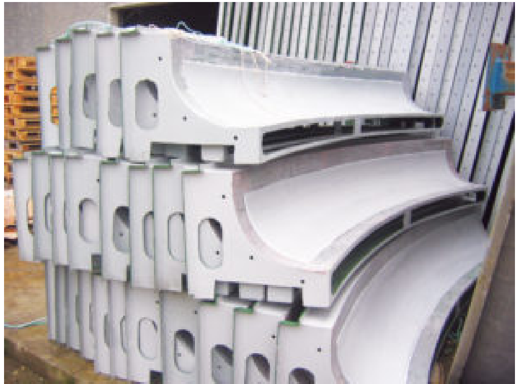
The fiberglass "base panel" sections eased installation of the tanks on site.
