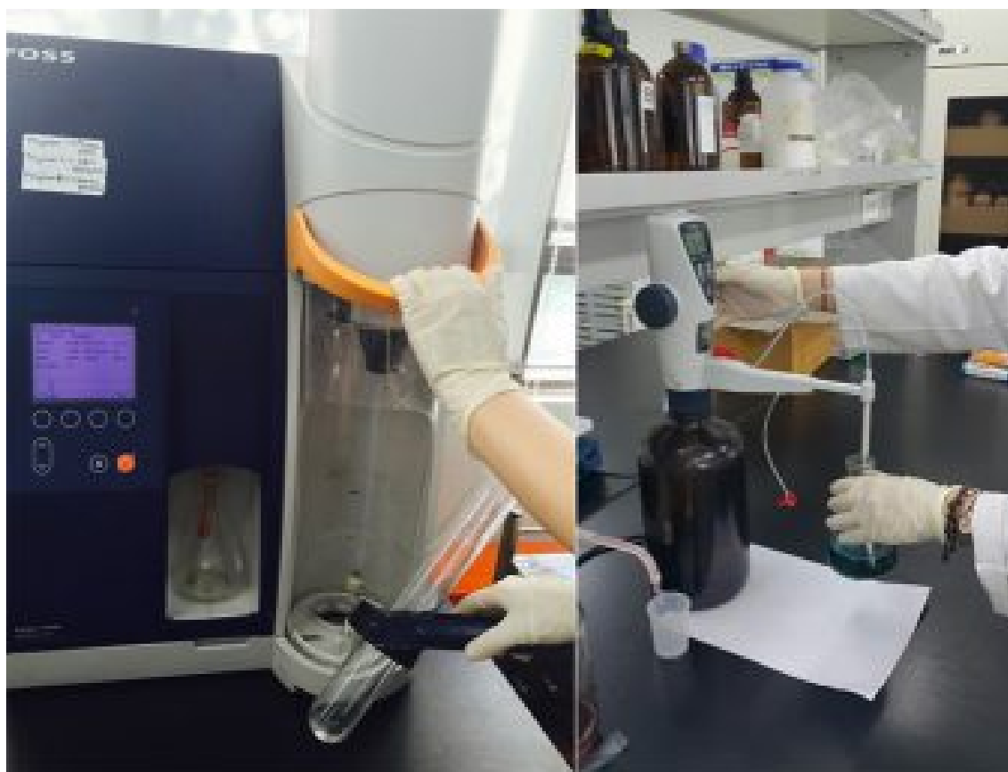
Analysis of crude protein by the Kjeldahl method for apparent digestibility coefficient.
