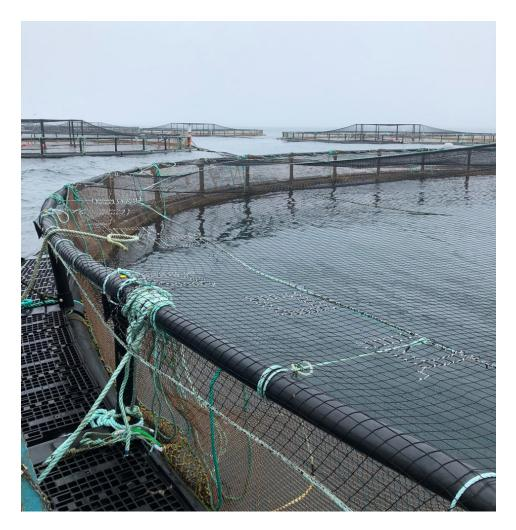
Net pens made of high density polypropylene, like these on salmon farms off the coast of Norway, retain strength better and last longer than nylon. Photo courtesy of Garware Technical Fibres Ltd.
