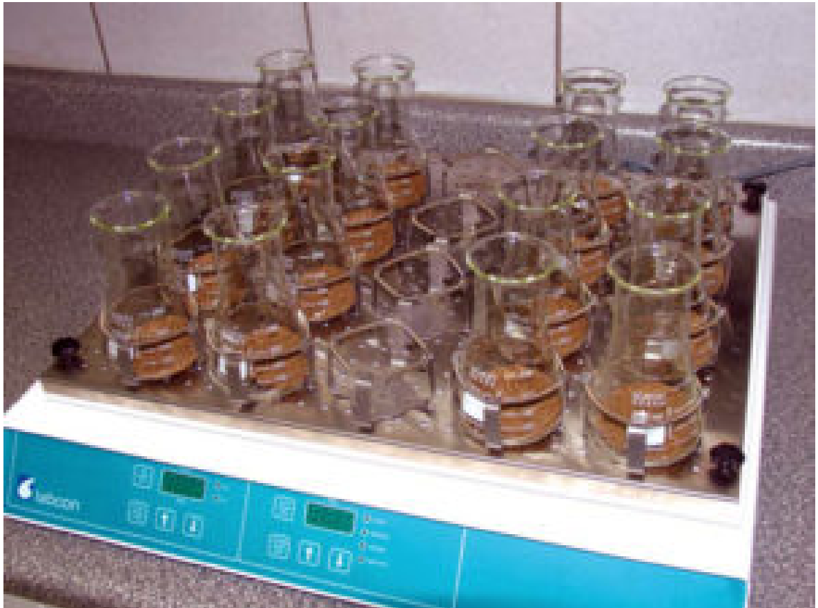
Feed samples are agitated to speed up the degenerative effects of water on feed pellets.
