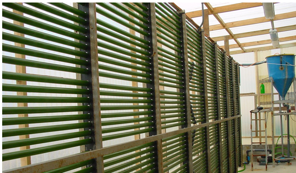
Automated, intensive algal production system.
