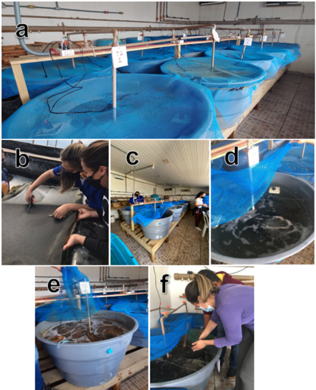
Fig. 2: Experimental units (a), artificial substrate management (b), artificial substrate installation (c), clear water (d), BFT system (e), and harvest (f).
