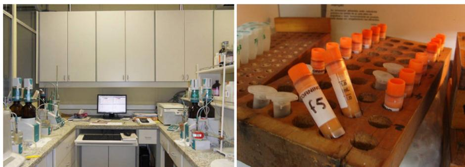
Left: View of the analytical station with titrators and central control software for pH-stat determination of protein hydrolysis at LAM-USP.
