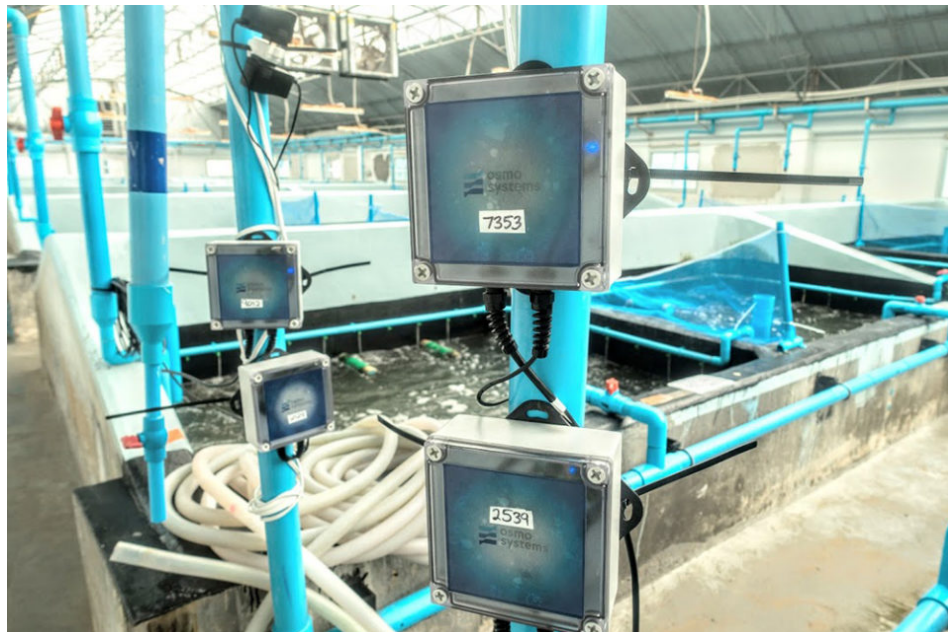
Prototype Osmobot system in place in an indoor RAS facility. Photo courtesy of Osmo Systems.
