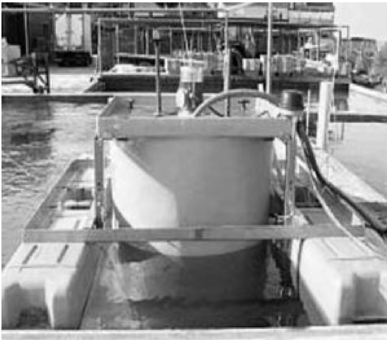
The new floating skimmer in operation during cockle purification experiments conducted by SMIDAP.
