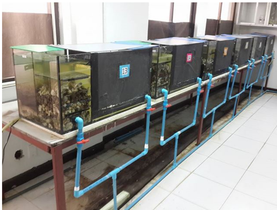
View of experimental setup, with each tank having its own water recirculation system.
