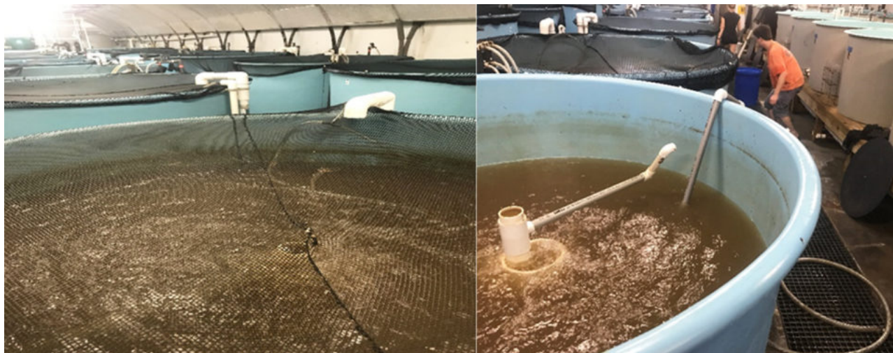
Fig. 1: Experimental 1-cubic-meter tank design. The tank on the right, partially drained, shows the airlift driven circulation system.
