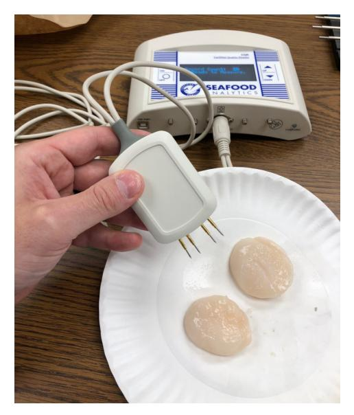
The Certified Quality Reader device has electrodes that when pressed against a specimen send an electrical signal through the animal. Photo courtesy of Seafood Analytics.
