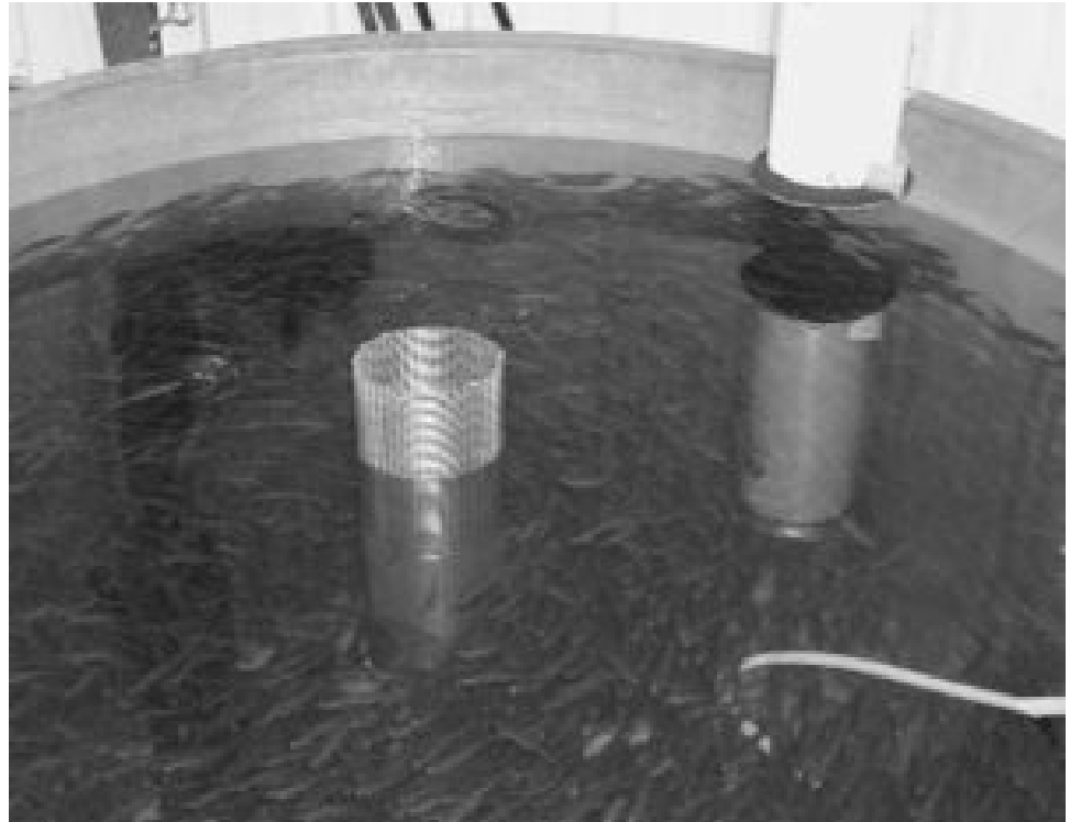
This culture tank has a microbubble oxygen diffuser for emergency use.
