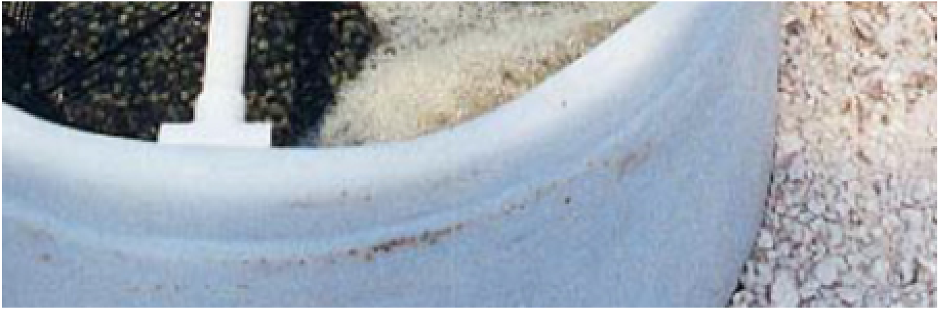
Stirring floating media within upwelling solids filter to release trapped waste for discharge through drain. Photo by Darryl Jory.
