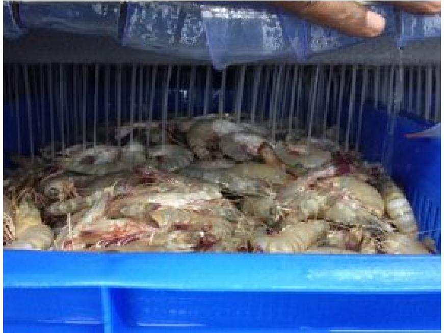
Brine freezing of shrimp in a shower of brine aqueous solution.
