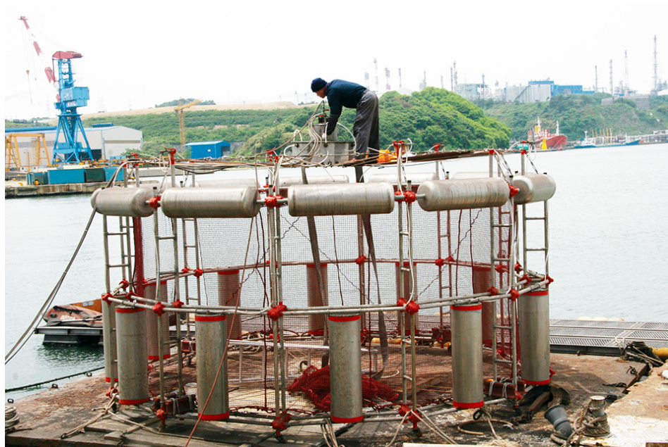
A worker checks the control station on top of a remotely operated submersible fish cage system.
